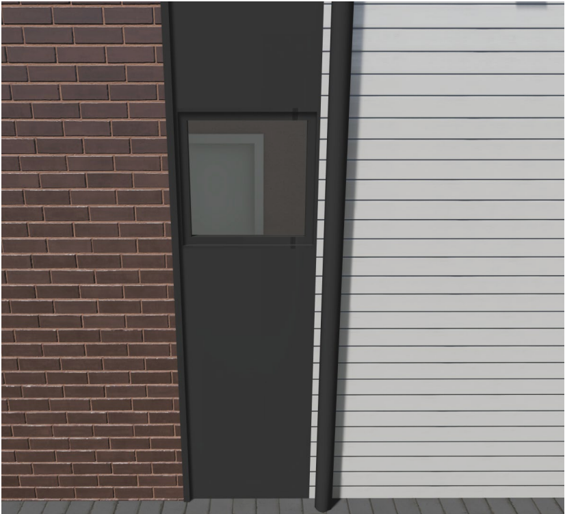
brick to panel to lap transition + gutter
