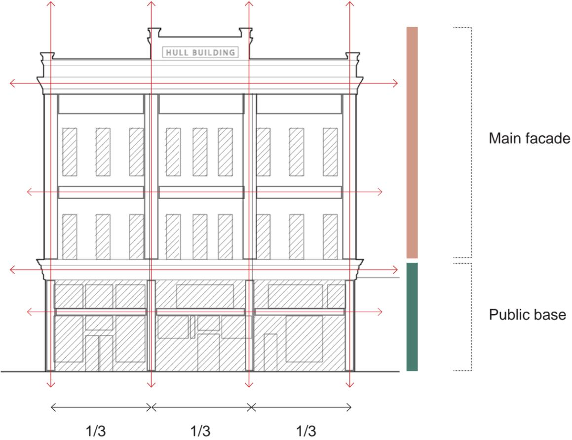
The Hull Building has a layered facade of vertical piers and horizontal spandrels. These layers are a woven arrangement. The windows are tall and generous in size.
