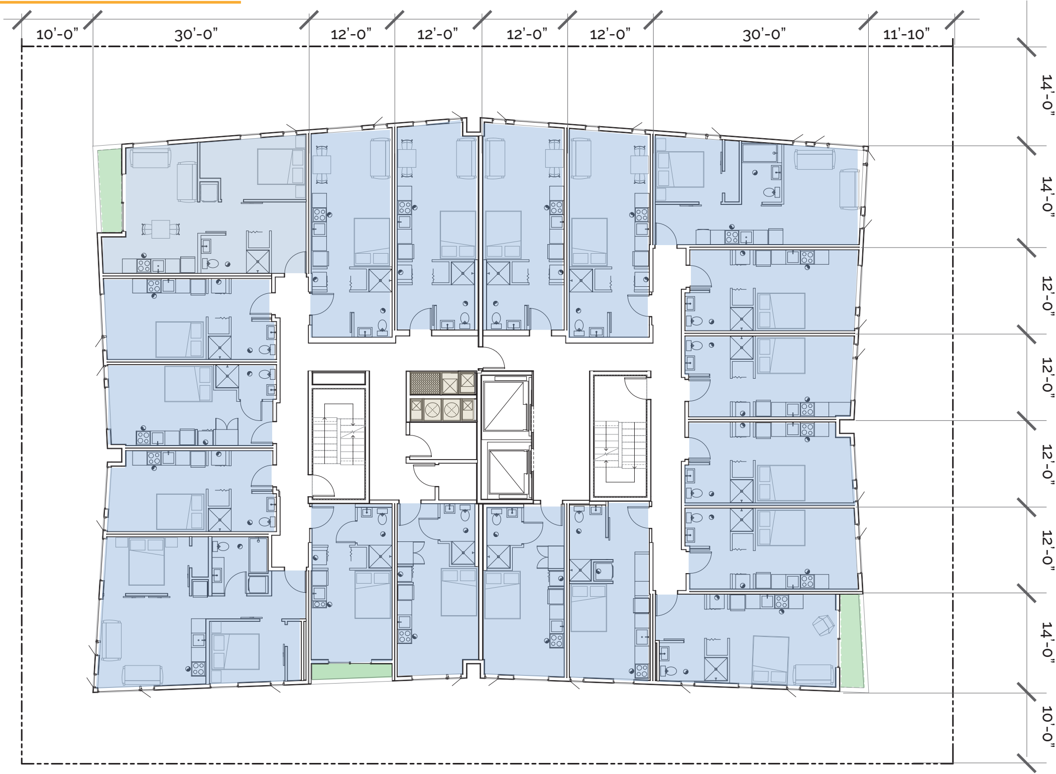
3rd, 5th, 7th Floor Plan Scale: NTS
