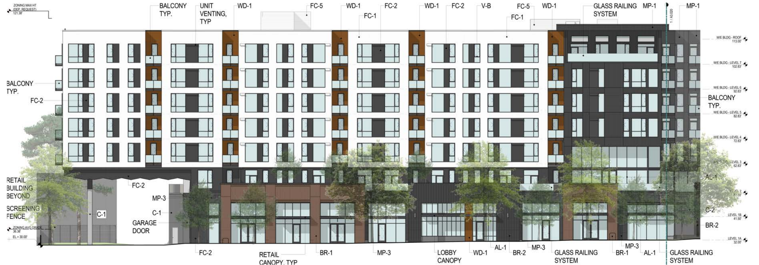
1 WEST BUILDING, SOUTH ELEVATION (NE 45TH STREET FRONTAGE)
