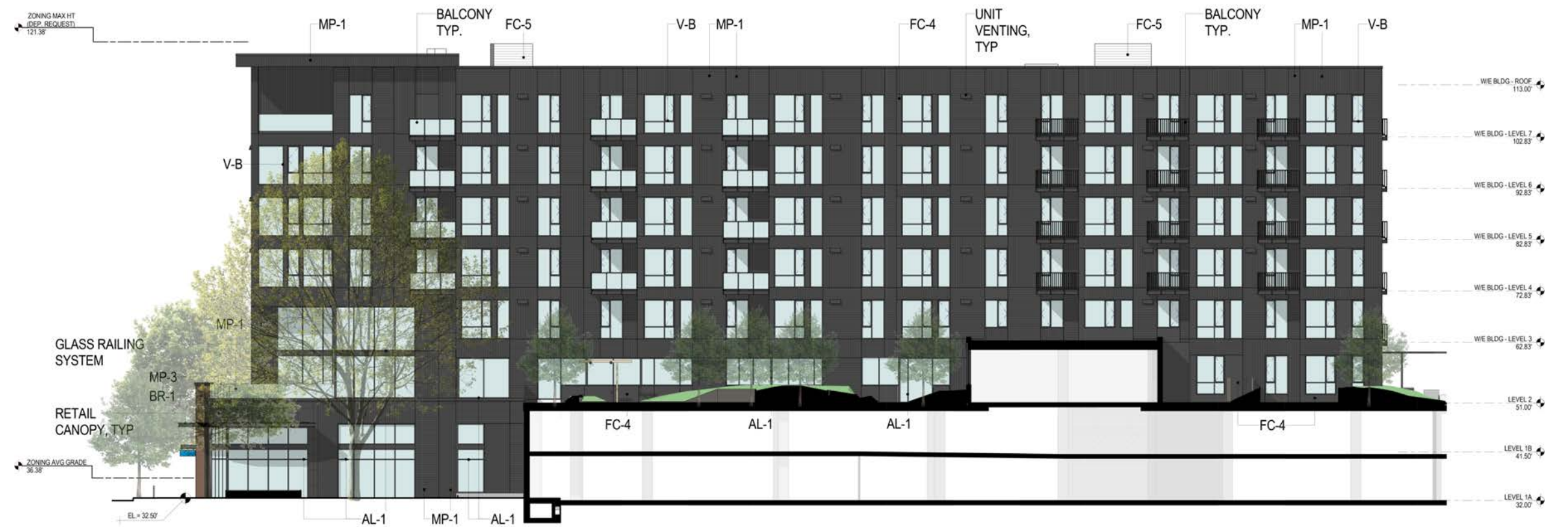
2 WEST BUILDING, EAST ELEVATION
