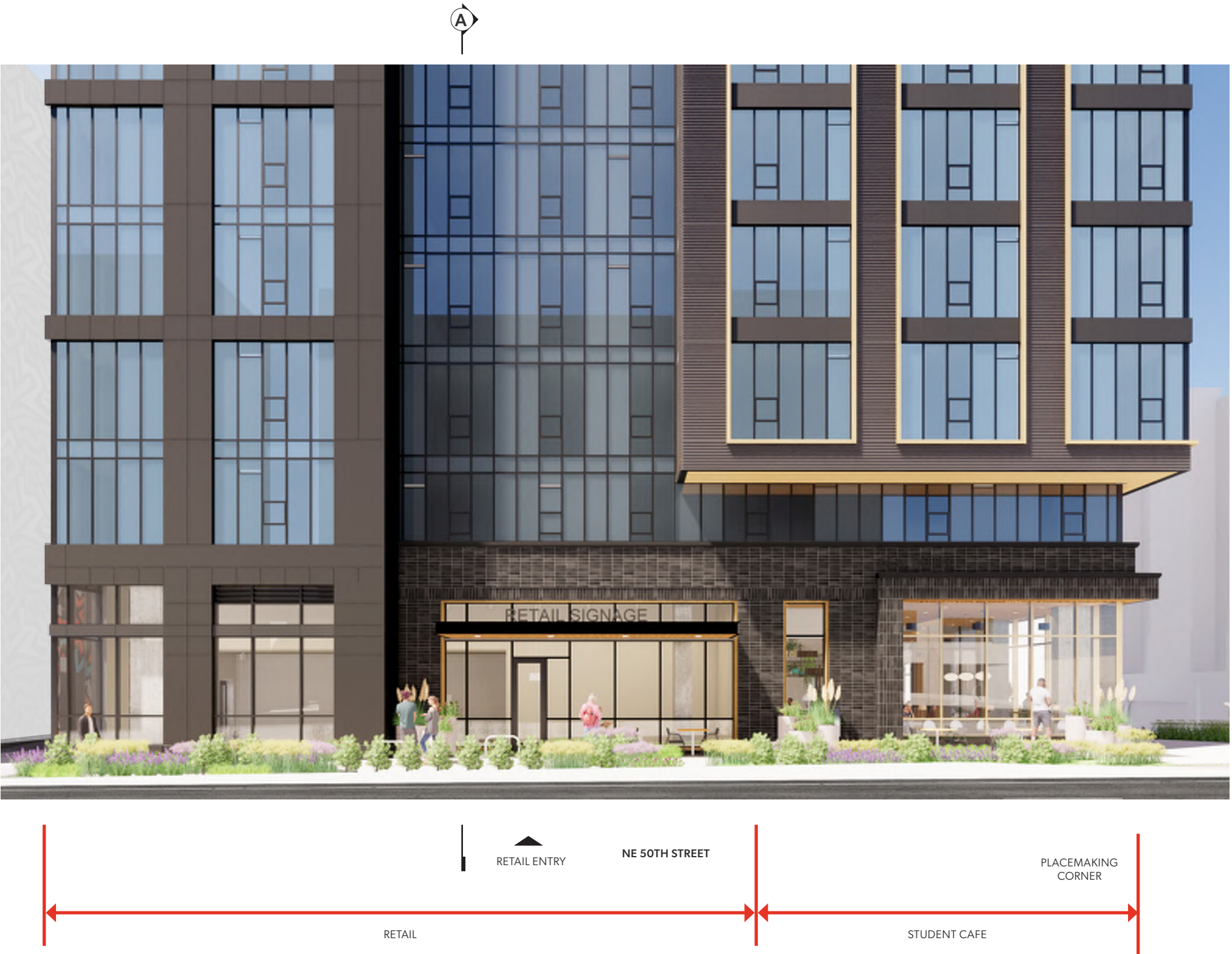
Detail elevation at NE 50th St. showing aligned metal panel system at alley and 50th corner and aligned brick podium with storefront infill at North Elevation.
