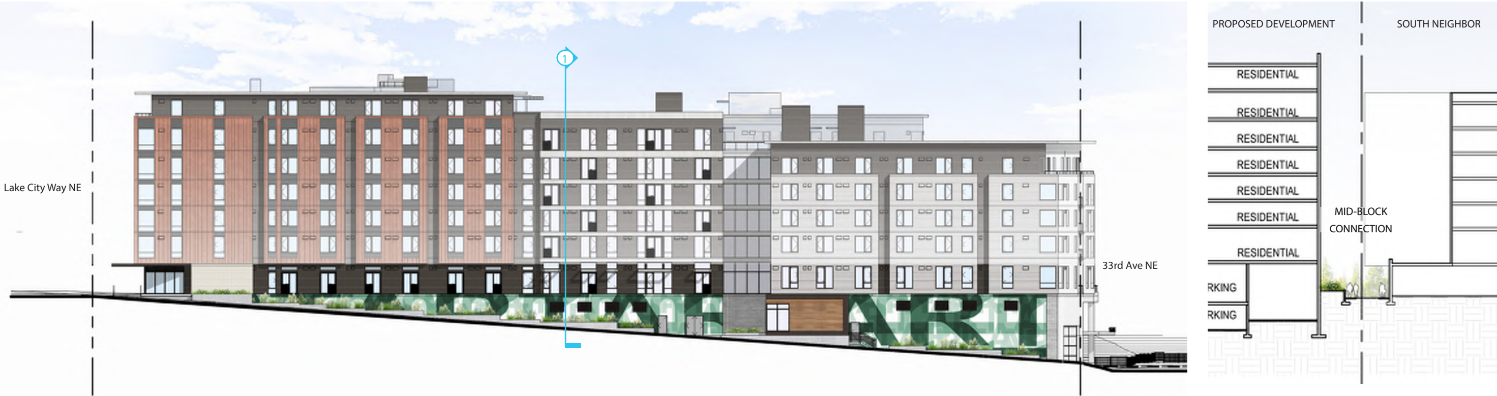
Figure 5: Elevation and Section showing mid-block connection. This passageway will be animated with mural arts on the wall, multiple types of lighting, planters, and Juliette balconies. Accessible slopes and landings will be provided along the route from Lake City Way to 33rd Ave NE.
