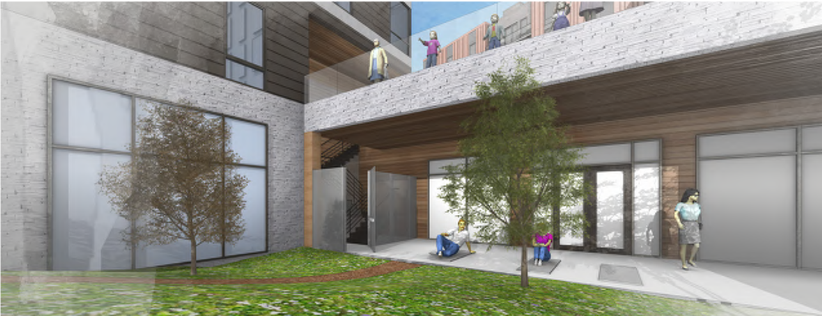
Figure 9: The perspective above illustrates where the stair connects the yoga deck to the courtyard level. A perforated metal gate provides security for tenants.
