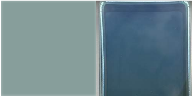
SG-1 | Spandrel Glazing Double Pane Insulated IGU with 4-sided silicon structural glazing, spandrel coating on #4 surface
