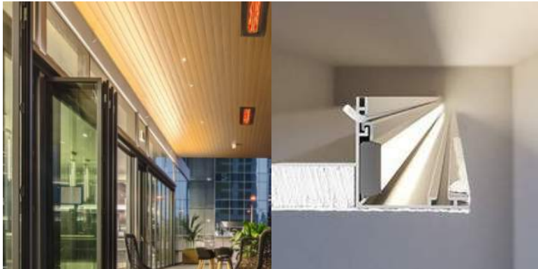
3 Linear Uplight at Balcony Soffits Linear cove light at balcony and L02 terrace soffits to create consistent soft wash lighting and warm glow visible from street.
