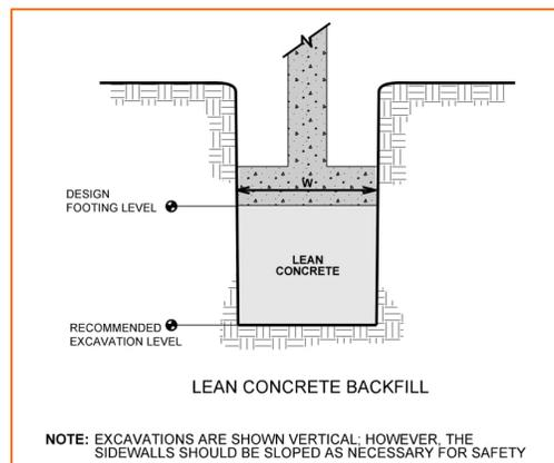
The subgrade soils at the base of the footings are anticipated to be silty, therefore disturbances of the subgrade soils from foot traffic during placement of formwork and rebar to cast the footing excavation are suitable, the contractor should consider over-excavating the footings by several inches and backfilling with lean concrete or crushed rock to preserve the subgrade condition.
